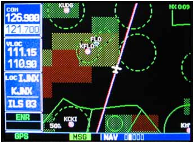
GNS 530 Datalink Screen shot of same weather. Notice the large blocky presentation of weather due to the lower resolution (36 sq. mi.), which might cause you to deviate much more than needed.
